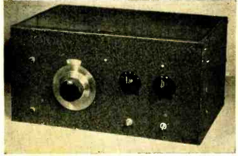
Twenty watts output on any desired frequency between 7000 and 7200 kc. with stability and a note comparable to crystal can be obtained from the "XEC," an exciter incorporating an electron-coupled oscillator of improved design.
