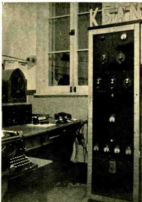
K5AN, Fort Randolph, Canal Zone, uses a T55 in the final with 150 watts input on c.w. and 100 watts on grid-modulated phone. Two vee beams are used, one aimed on New York and the other on San Francisco.
